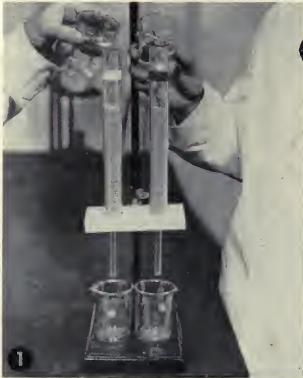
CONDITIONED SOIL LETS ALL THE WATER THROUGH. —Soil in the tube at left has not been treated; at right, treated soil. Using the same amount of water and soil, photo No. 2 shows how the untreated soil obstructs the passage of water.
